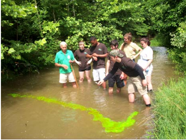
Using dye to calculate flow rate and patterns.
